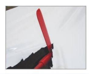
as the grain is being taken out from the bags, the extractor moves forward, cutting the bag automatically and progresively with a coulter intended for that purpose. There is no need of a worker participation to cut the bag. The top capacity reaches 180 t/h.
