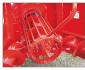
The augers are put into the bag and they carry the grain to the central collecting auger - with a diameter of 340 mm - which takes the grain to the loading point.
