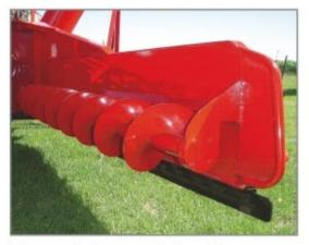
It is composed of two augers onto two mobile screens whose angle is modified by means of hydraulic cylinders.
