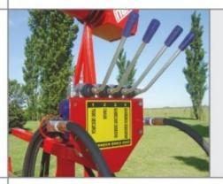
The extractor has a hydraulic distributor with four valves to command all the hydraulic moveme
