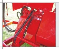
The unloading augers driving action is done by means of a cardan control of 6 ripple marks working at 540 rev/min. It is advisable that the p.t.o. connection would be independent from the gear box connection to avoid unnecessary stops of the machine as it moves forward.
