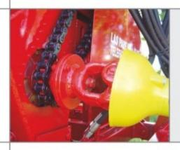
The transmission is protected by a detachment device by means of fuse screws in the cardan control. The minimun power the tractor should have is of 80 HP.
