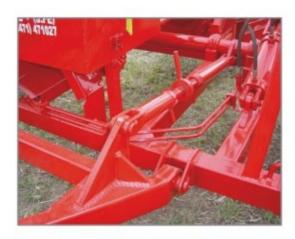
It has a robust tubular chassis with 6.50 - 16 tyres and with a tilting shaft and an articulated lance regulated by screw.
