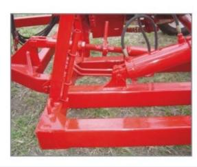
This articulation allows the shifting from the trasnport position to the work position just by a hydraulic command. The machine keeps horizontal in any position.
