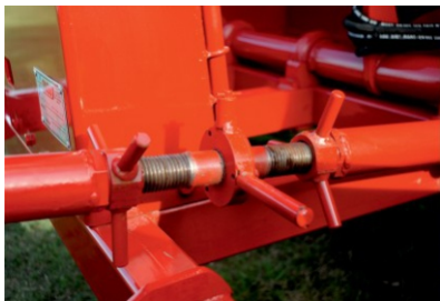
Adjustable articulated chassis and drawbar.
