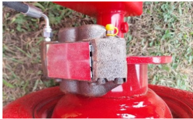
Hydraulic disc brake system.
