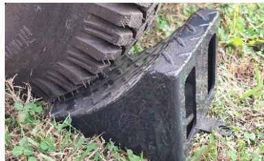
Wheel chocks to secure the machine when stationary.
