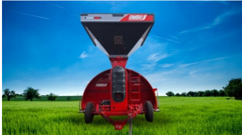
Machine in working position with rear support legs for tractor removal
