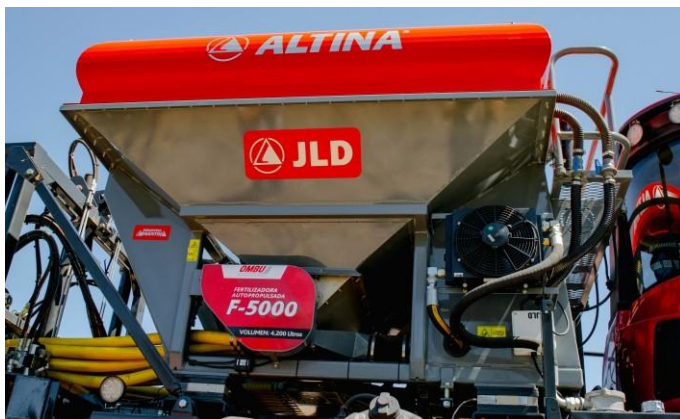
Stainless steel hopper. Pressurized with agitator and anti-clog sieve. It includes a solid flow divider for even distribution of material within the hopper. It prevents spillage outside.
