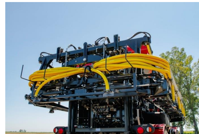
2 stainless steel dispensers with 3 sets of dosing rollers and electro-hydraulic drive.
