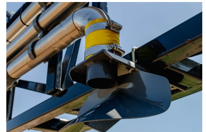
Diffuser Nozzles: up to 18 ALTINA brand stainless-steel diffuser nozzles for total coverage distribution of solid products.
