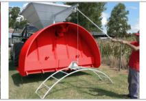
Perch system to lift and place Folding bottom for cleaning. the bag.
