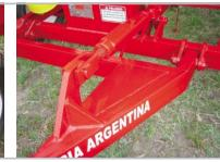
Manual register to leveling the drawbar of the bagger with the tractor.
