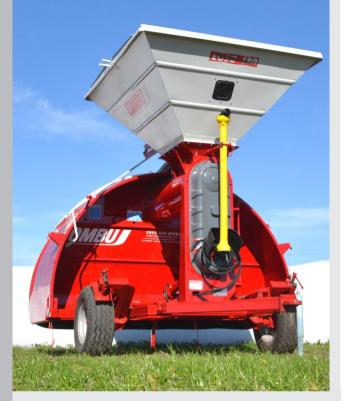
Its upper hopper permit a constant grain flow to the bag increasing the working efficiency and reducing the O2 percentage that goes into the bag.
