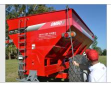
The roll over tarp system of the CRV grain cart has a lower profile towards the combine's unloading tube. Easy operation
