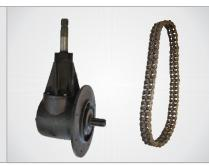
The transmission of the CRV grain cart is made by a double ASA 80-2H chain with a self- adjustable chain tensor. The gearbox has self – lube bearings and is located underneath the unloading tube and bringing direct transmission to the augers. This transmission is protected by a high impact fiberglass cover.
