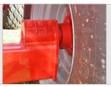
Robust with detachable axle spindles. The axle can be moved from its standard potision to vary the loading distribution. This procedure doesn't affect the functioning of the scale in case it was placed. Electronic scales are optional.
