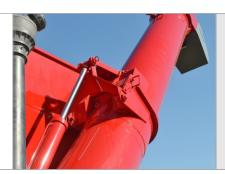
For the unloading tube opening has a 3 " diameter cylinder and the coupling system of the upper/lower tubes prevent the loss of grains.
