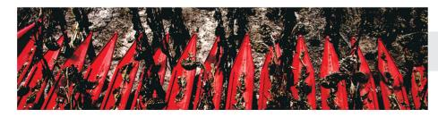
**Cutter bar:** commanded by an oil bath gearbox which produce alternative moves, includes welded and forged pan supports and 70-30-6 blades riveted to the bar.
